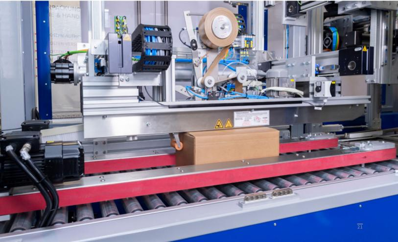
also lets you choose between different sealing types: U-shaped for standard parcels (with optional pull strip), C-shaped for extremely flat cartons, or T-shaped for the optimum sealing of heavy cases. It should also be pointed out that water-activated tape is theft- and tamper-proof and that the recipient can dispose of it, together with the box itself, as waste paper.
